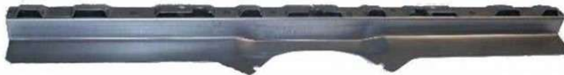
Superior reinforcement back door
