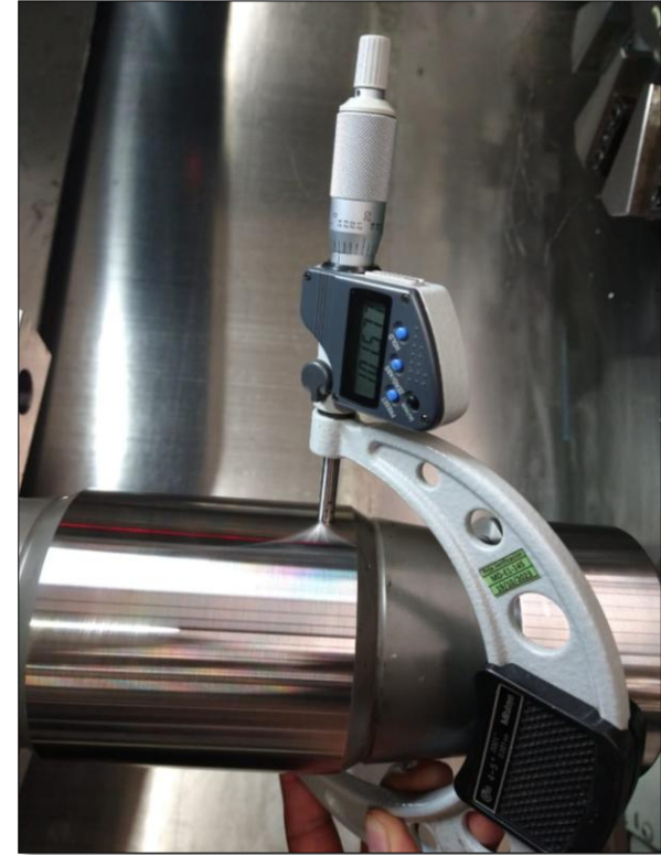
Hard turning (60-62 Hrc) with .020 mm tol.
